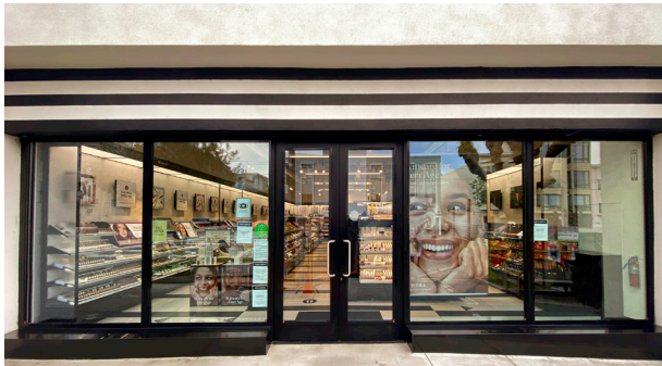
Bronze ArmorPlast® system with full frame on the windows and surface mount on the doors.
