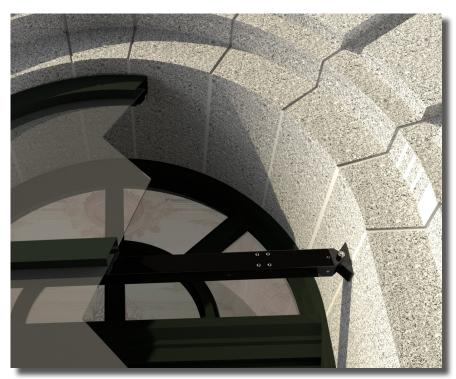
J-Series compression frames provide an extremely secure base structure on which to mount any Riot Glass® ArmorPlast® window product without drilling anchor holes or adhesives that would leave marks on the surrounding stone surfaces.
